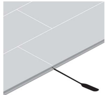
14. Place tool between two boards at end seam to "unlock".
